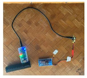
This picture shows Dongle plugged into a USB power source and connected to a 3 servo VR Magic Timer using the 2.5mm Stereo type cable. It is very important to make sure the connecting cable is fully plugged in at both ends.
